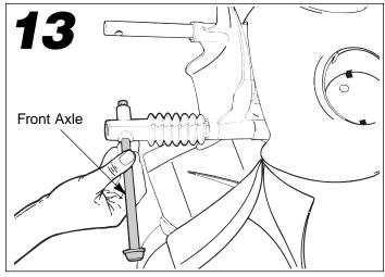
Slide the front axle through the hole in the shock halves and handlebar.
